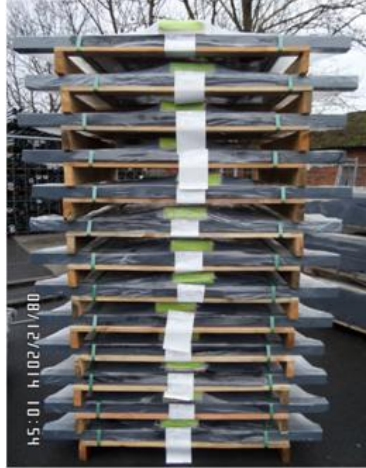
Picture 2: Position of the product identification label
